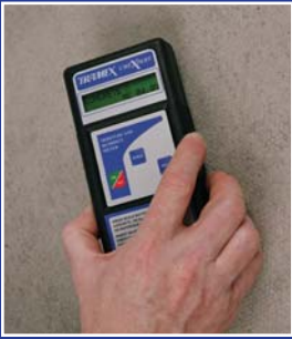
% Moisture Concrete Slab
