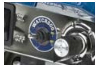
WatchDog Pump Protection System prevents dry pumping damage.
