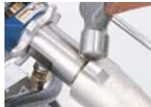
Endurance Pump with hammer access inlet valve.
