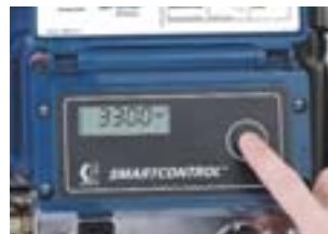
Digital display with pressure readout, job/lifetime counters, and AutoClean timer.
